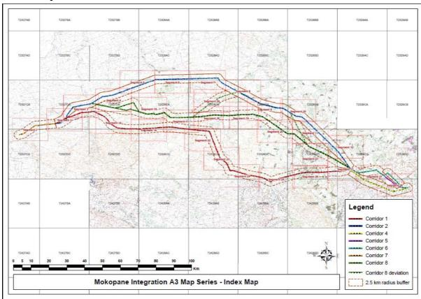
Figure 1- The Mokopane Integration Project with the proposed sites for the Mokopane Substation and various power line corridors in the Limpopo Province of South Africa.
